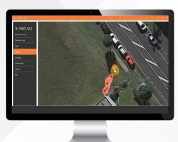
X-PAD VU allows an easy analysis of activity data from one or more EZiCAT cable locators. Simply download the data via Bluetooth to see how the data survey was conducted and issue reports of the collected data. The software can be used with all EZiCAT i700 as well as previous models of EZiCAT i600 Series.
